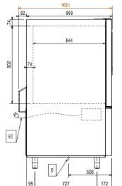
Drain Electrical inlet (power)
